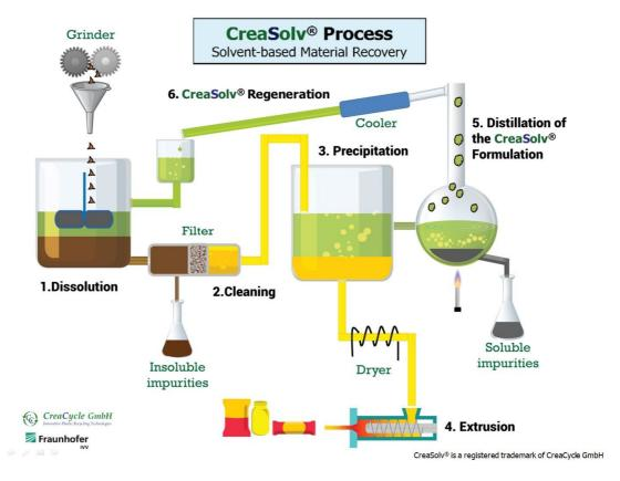
The process concept is relatively simple and can be compared with a washing machine on a molecular level (polymer chains in comparison to textiles) that can remove imbedded unwanted impurities or additives (e.g. flame retardants or softeners which are actually considered as POPs - Persistent Organic Pollutants) or other materials in plastic composites (e.g. metals, fibers, etc). For more information please check: CreaCycle GmbH – CreaSolv® Process - https://www.creacycle.de/en/the-process.html
