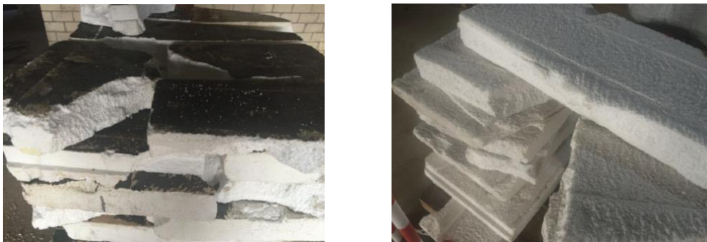
Figure 3. EPS flat roof boards with bitumen leftovers before and after treatment [18].
