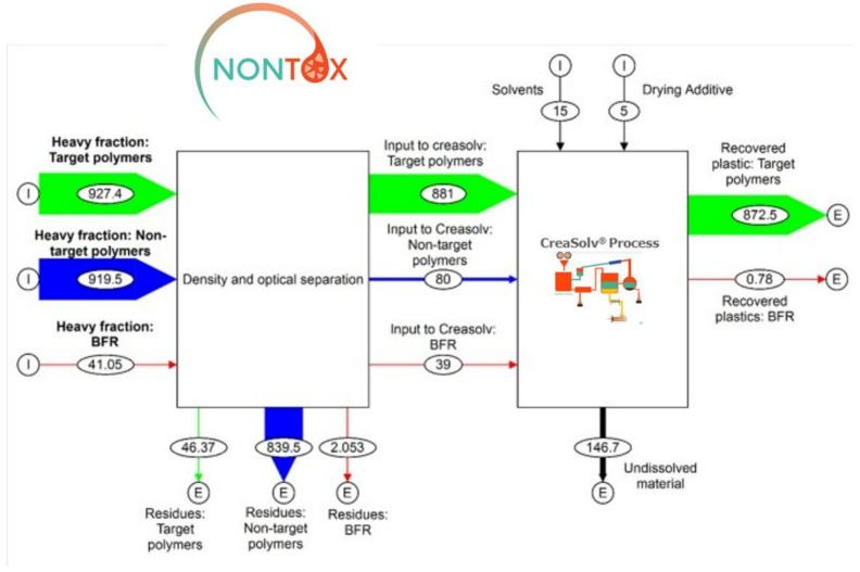
Quantitative flowsheet of the CreaSolv® Process with prior sorting process. Each flow is reported by indicating the related amount in terms of target and non-target polymers, and BFRs content. Data are reported in kg and refer to 1000 kg of input to the CreaSolv® Process. I = import; E = export. Source: Fraunhofer, 2021, EC-JRC, 2018.
