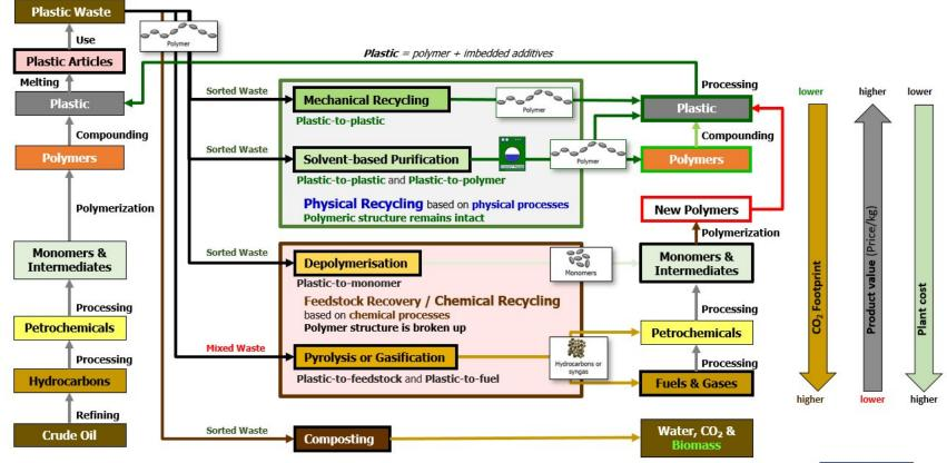
Solvent-based Purification/Dissolution Recycling allows the REUSE of the Materials Plastic & Polymer with lower CO<sub>2</sub> footprint and investment cost than chemical recycling. It can separate composite materials, embedded additives & hazardous impurities, as well as polymer degradation products, thus enabling unlimited recycling cycles.
