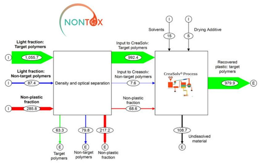
Quantitative flowsheet of the CreaSolv® Process with prior sorting process based on optical and density separation. Each flow (light fraction, input to the CreaSolv® Process, and recovered polymers) is reported by indicating the related amount in terms of target polymers, non-target polymers and non-plastic fraction. Data are reported in kg and refer to 1000 kg of plastics in input to the CreaSolv® Process.
