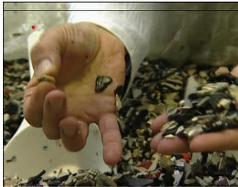
plastic waste. The estimated yearly volume for Germany is 200.000 tonnes and the waste-handling is costly. Straightforward melting of the colored mixture is technically not feasible because dangerous toxic degradation products could be formed.
