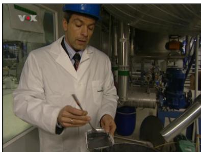
**Andreas Mäurer:** Here we are at the lower part of the plant. This is the bottom area and the discharge unit of the vessel. The compound exits here and is collected in this drum. You can see that it has already cooled down to room temperature. It is then a bit more viscous. When it leaves the reactor at higher temperature it behaves like honey/syrup. Then it has this consistency here. In a real plant there will be an extruder directly below here and the compound will be processed.
